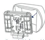
Remove the sounder interface module from the base.
